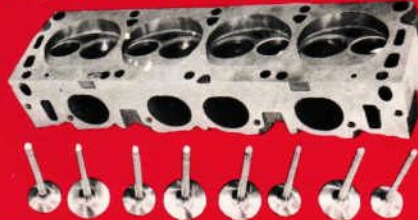
427 Tunnel Port Head w/ Lightweight Valves
