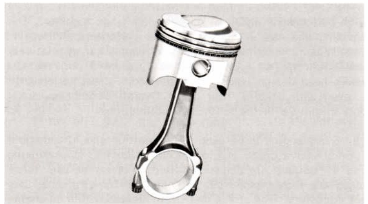
Figure 3 — Impact-extruded Piston and Special Connecting Rod
