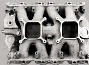
Ford 8V single plane manifold for Tunnel Port heads.
