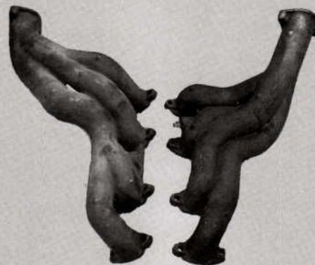
Ford Police Interceptor exhaust manifolds for street use, #'s C3AZ-9430-E (R), C3AZ-9431-E (L).
