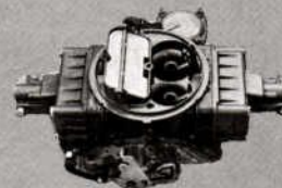
Ford Center Pivot-type carburetor for use on 4V manifolds.
