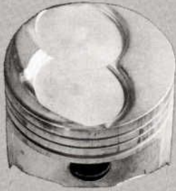
Pop-up style high compression piston for 427 and 428 blocks.
