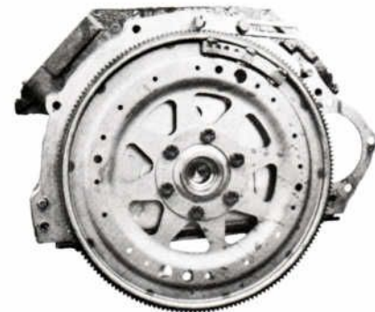
Figure 17 – Balance Weight on 428 C.J. Flywheel
