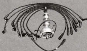
Hi-Per Dual Point distributor for all 390, 406, 427 and 428 engines, #C0AZ-12127-L.
