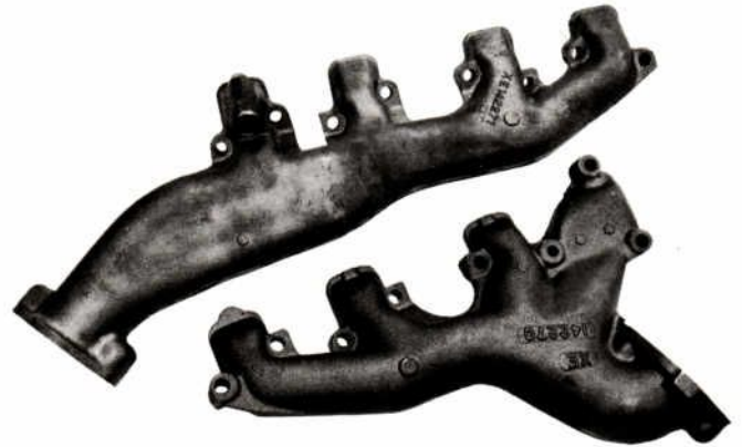
Figure 14 – New, Low Restriction Exhaust Manifolds
